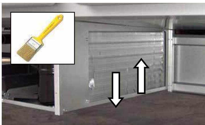
Fig. M Detail of the condenser; direction of cleaning
