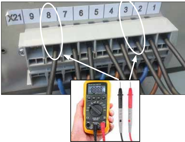
Fig. 2 Insert the tips into the terminals indicated
